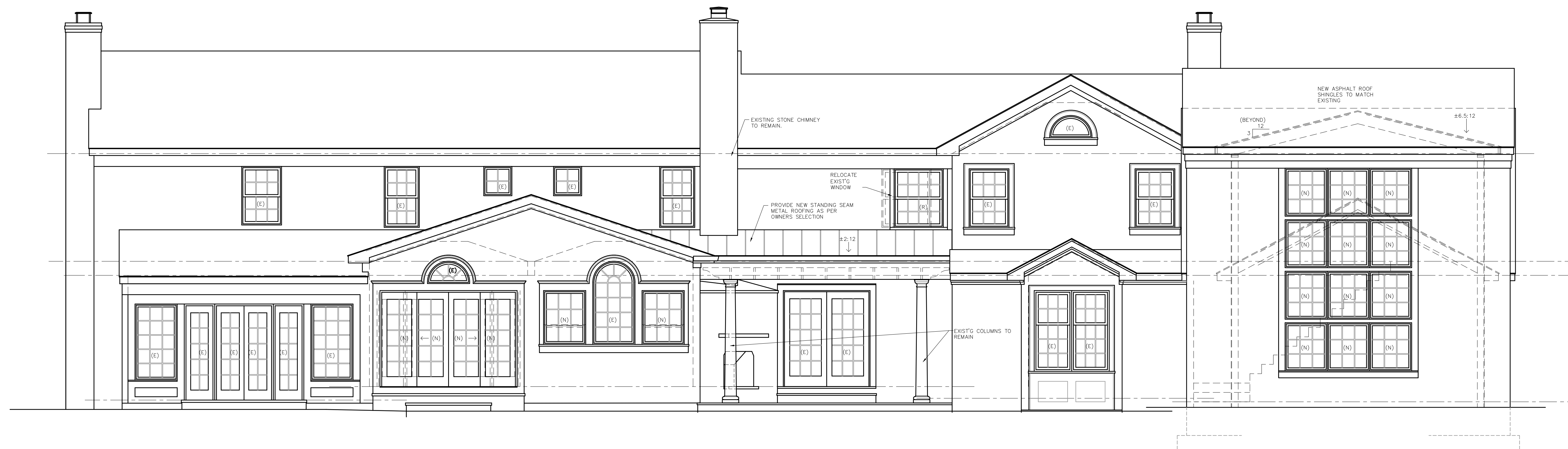
REAR ELEVATION SCALE: 1/4" = 1'-0"
