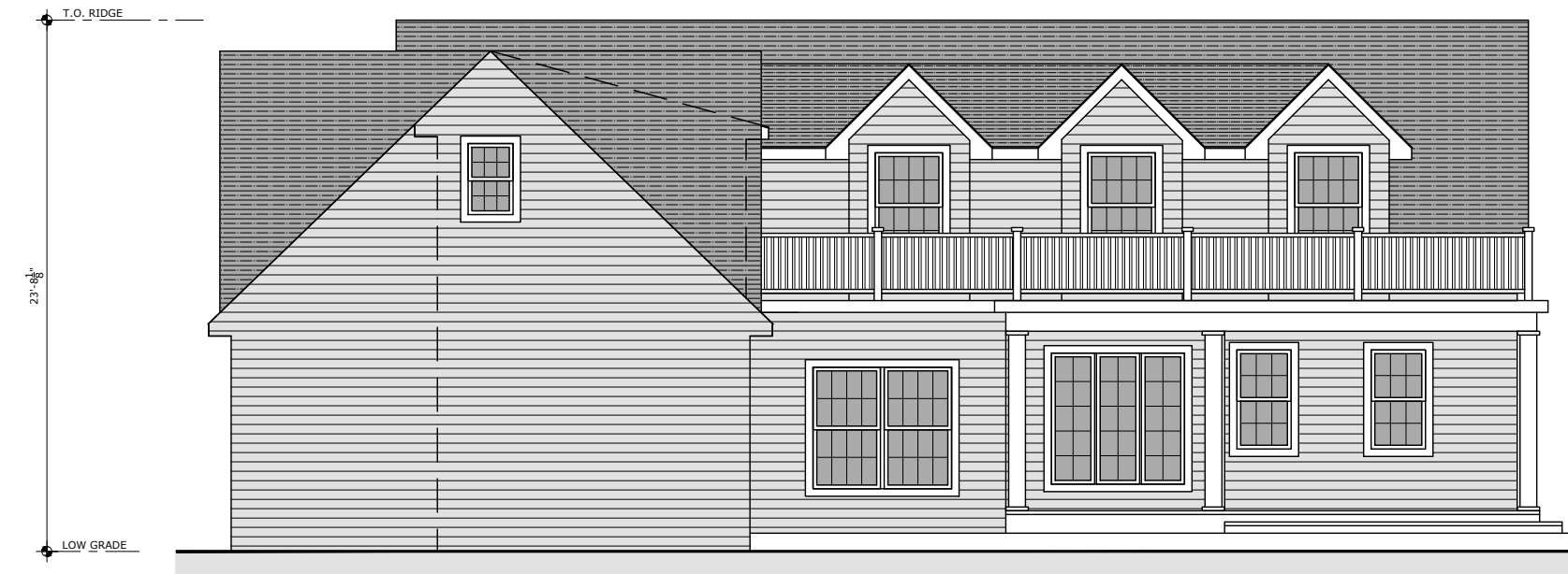
5 LEFT SIDE ELEVATION 1/8" = 1'-0"
