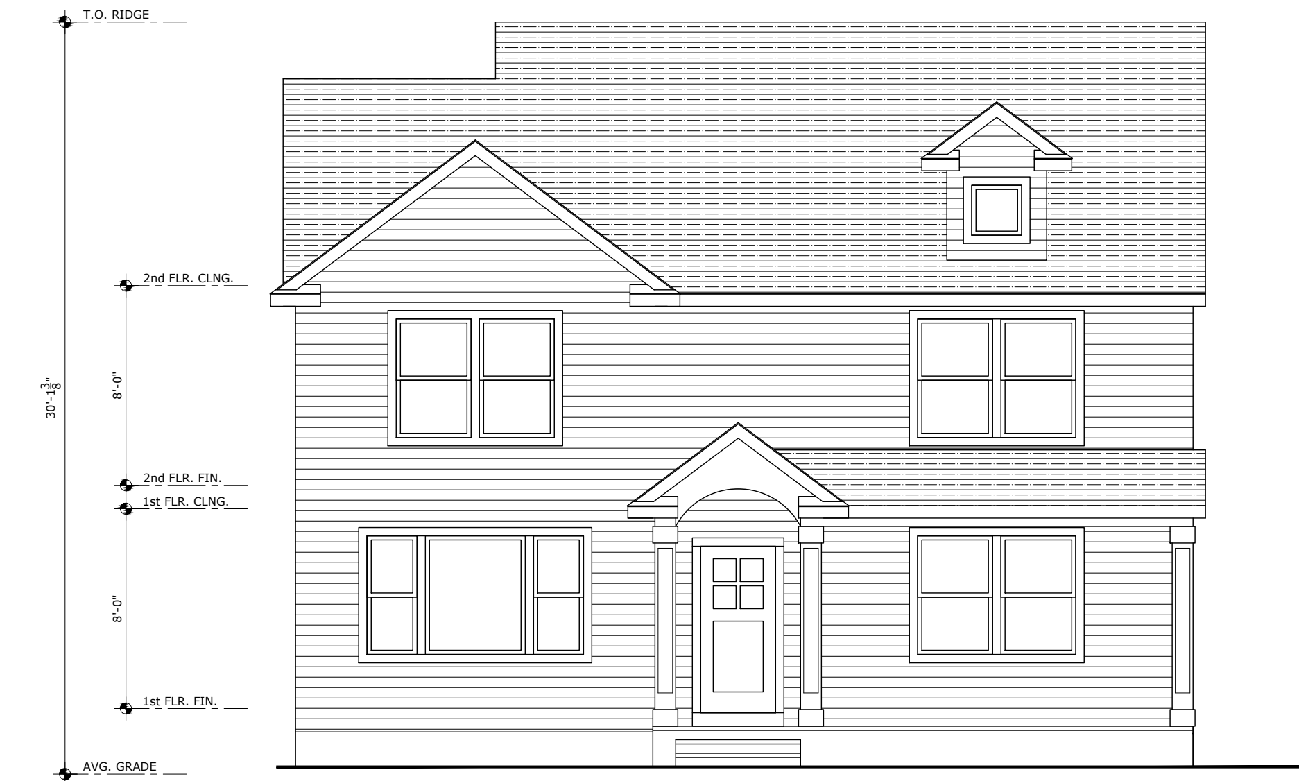
3 A2 FRONT ELEVATION 3/16" = 1'-0"
