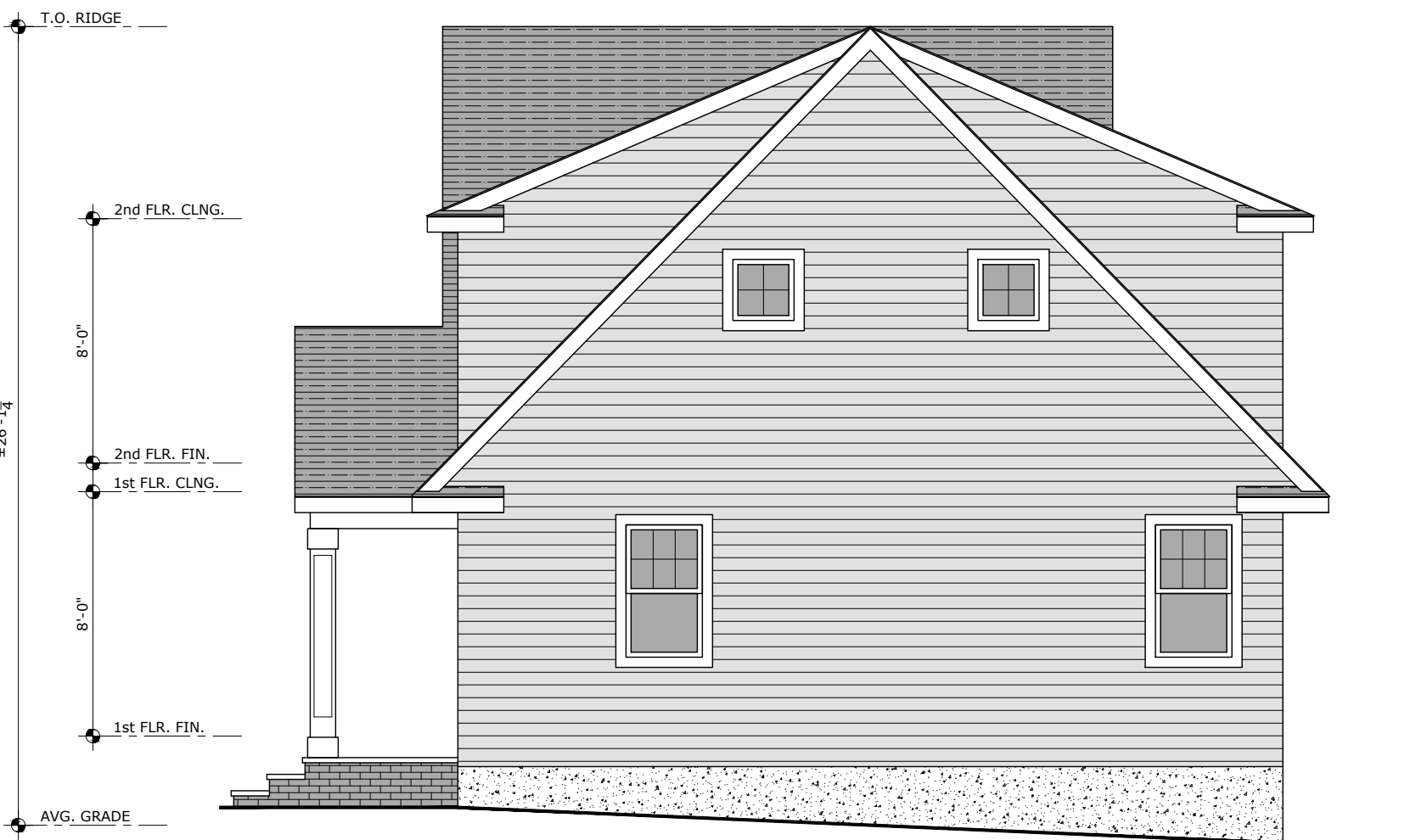
4 A2 RIGHT SIDE ELEVATION 3/16" = 1'-0"
