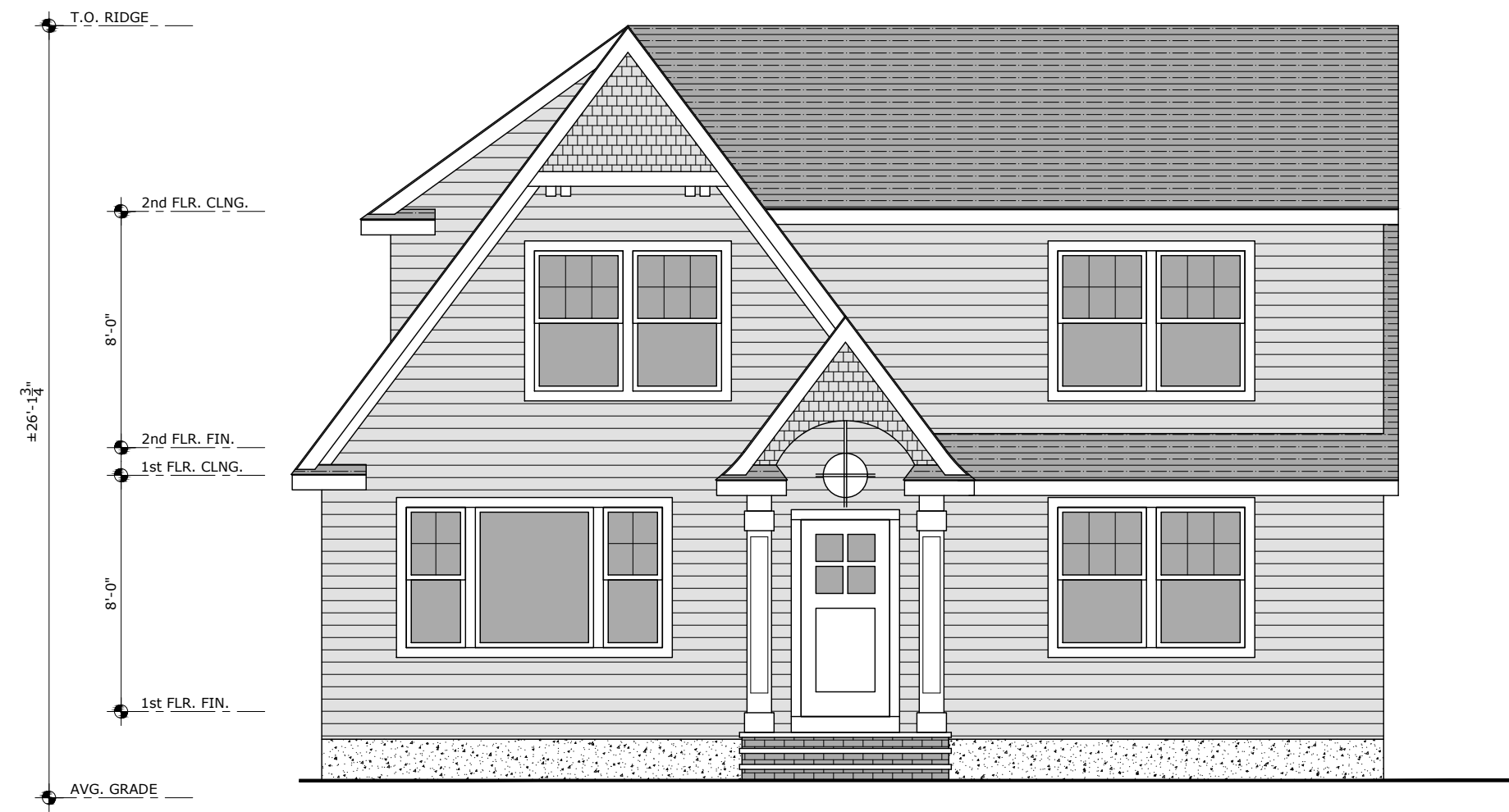
3 A2 FRONT ELEVATION 3/16" = 1'-0"
