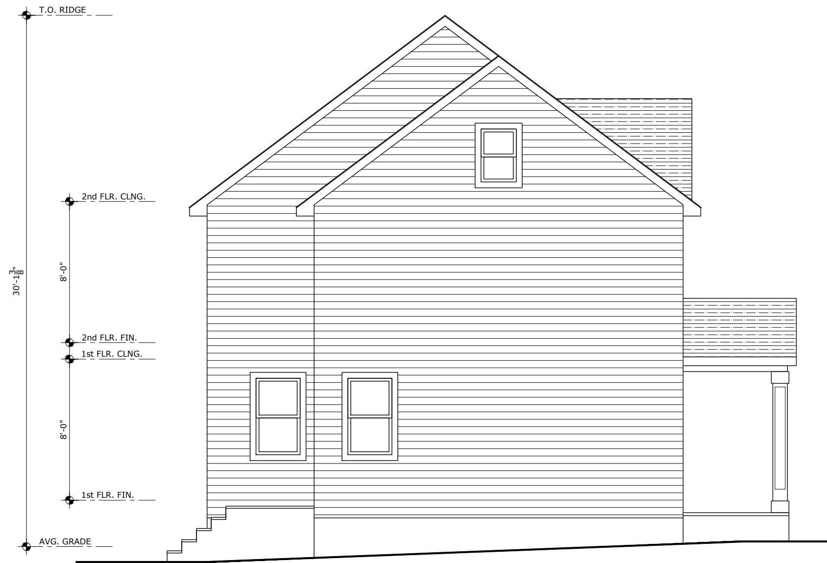
6 A2 LEFT SIDE ELEVATION 3/16" = 1'-0"
