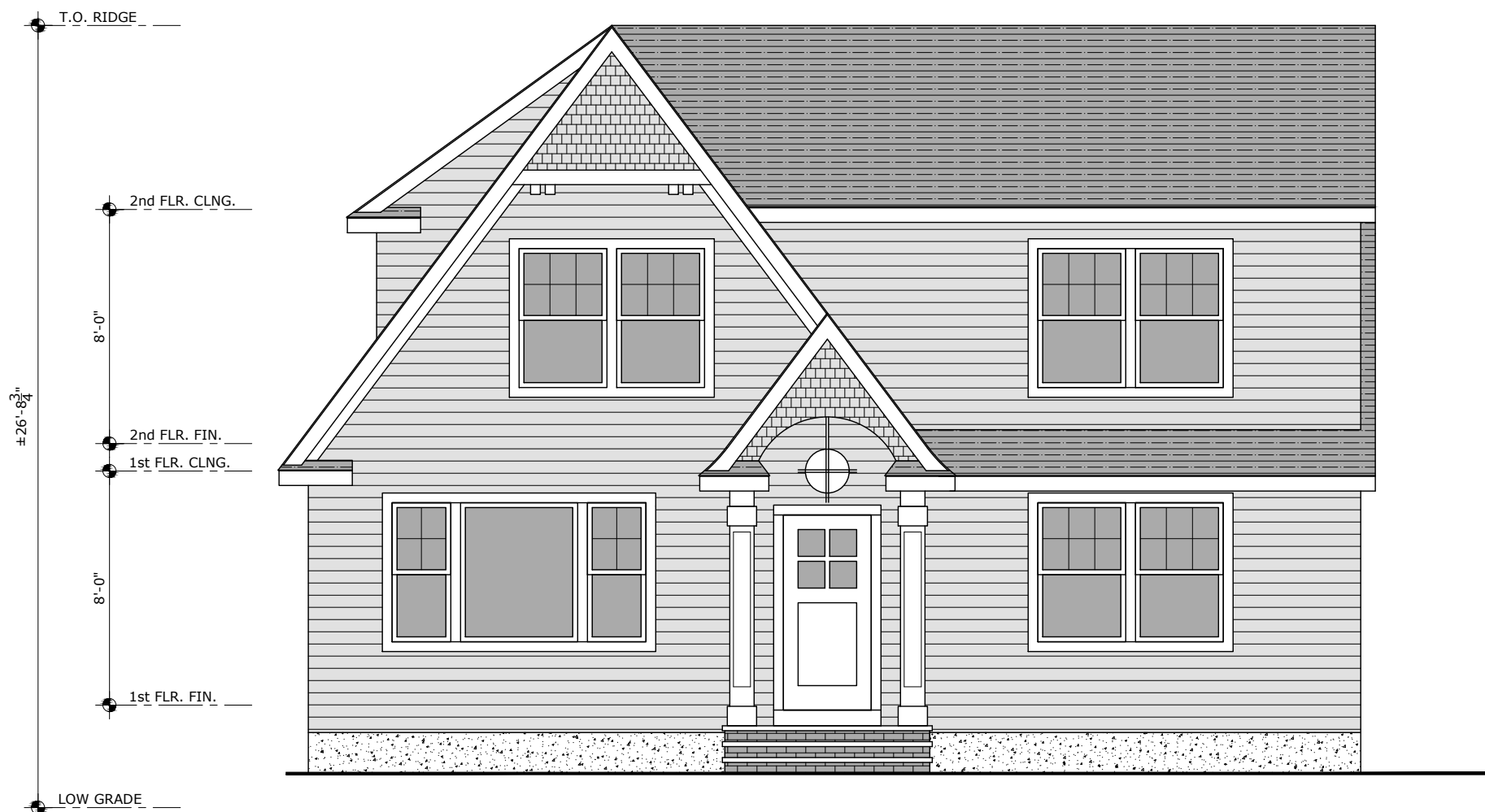
3 A2 FRONT ELEVATION 3/16" = 1'-0"
