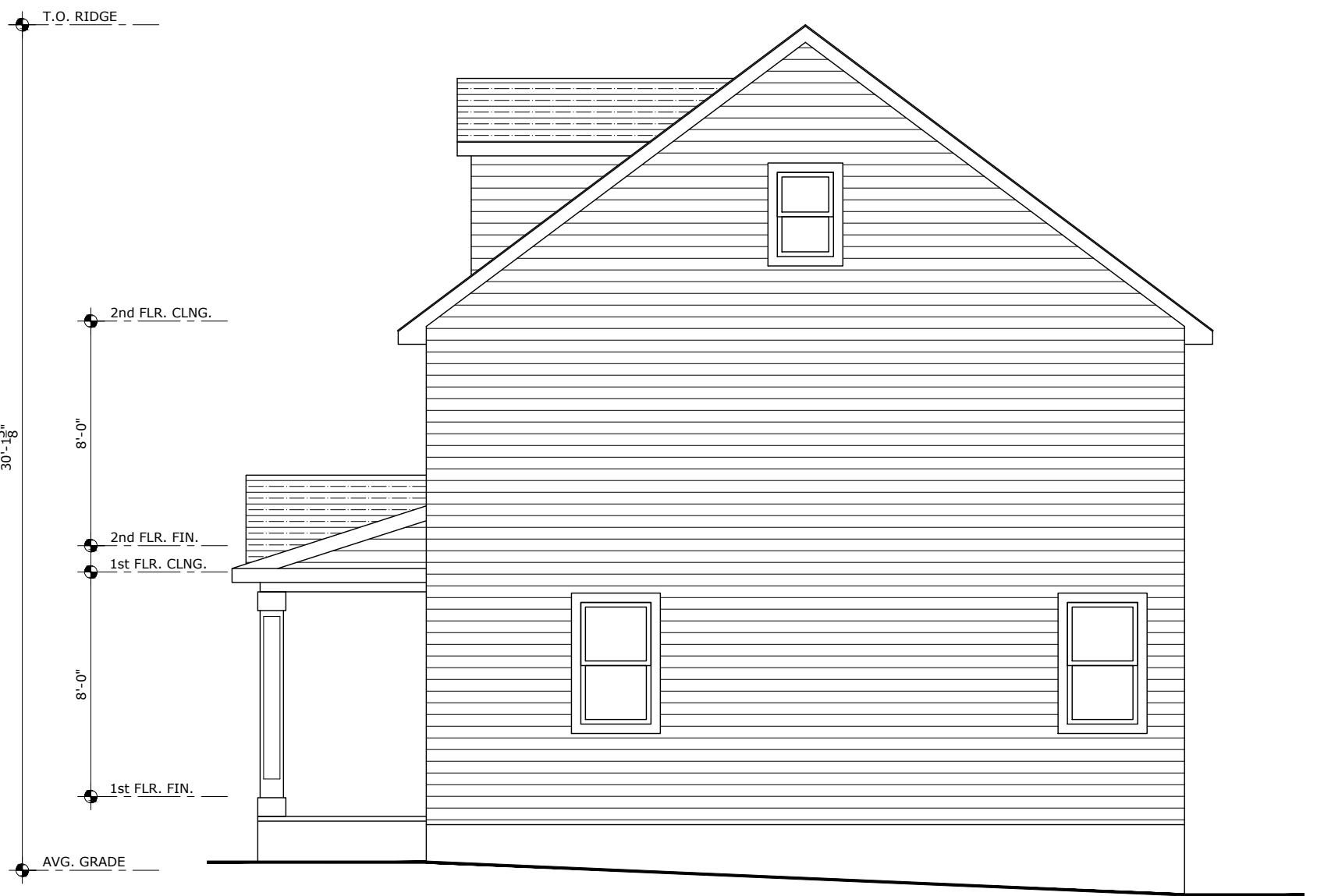
4 A2 RIGHT SIDE ELEVATION 3/16" = 1'-0"
