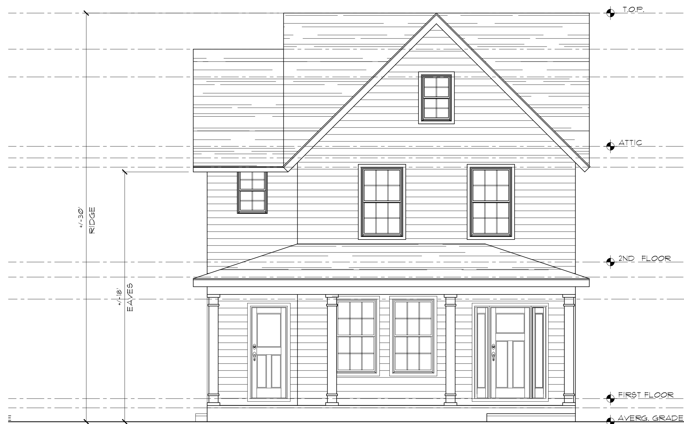
10 FRONT ELEVATION SCALE: 1/4" = 1'-0"
